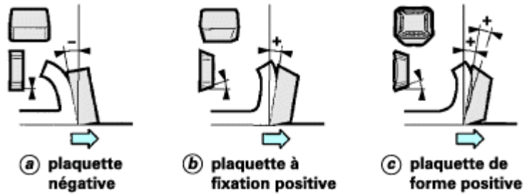
Figure 15 - Types de plaquettes de fraisage
